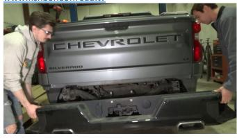
Remove the sensors and sensor wiring harness. Remove the license plate bracket and lights. Remove license plate lights. Remove the exhaust caps.
