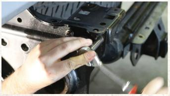
Install the mounting brackets using the remaing factory hardware, and the included 2 larger bolts, washers, and nuts using a 13mm socket.
