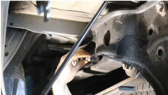
Remove both of the shown brackets with a 12mm socket.
