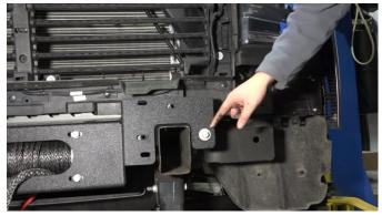
Install the bumper brackets with the remaining factory hardware and the included hardware with a 17mm socket.
