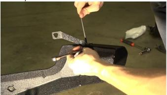
With a 3/8" drill bit, drill out the bolt hole shown below.
