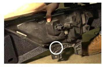
Loosely install your fog lights into the bumper using the M8 25mm, 30mm, and 35mm bolts using a 13mm socket. These bolts and washers are locations specific. The 35mm bolt secures the drilled hole, the 30mm secures to the fog light bracket, and the 25mm secures to the inside of the bumper.
