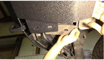
Reinstall the factory bolts with a 15mm socket.
