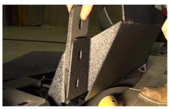
Using tape, adhere the two factory tow hook nut plates into the shown slot so that it doesn't slide around during installation.
