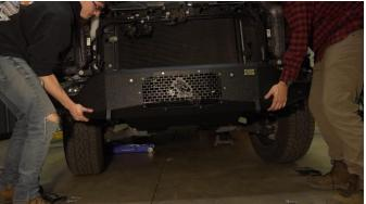
If you do not intend to run a winch plate, insert the spacers in between the bumper and bottom of the frame at this time.
