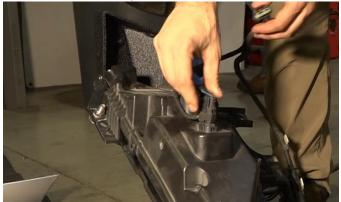
Install the included foam paddings onto the 2 mounting brackets, and the bottoms of the d-ring mount reinforcements. If your vehicle does not have a winch plate, place the remaining foam on both sides of the two included spacers. If you plan on installing Fishbone's Winch Plate Adaptor Kit, place the remaining 4 pads on both sides of its mounting locations, which lay between the frame skid plate.
