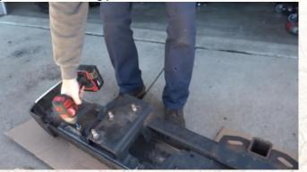
Push out and remove the license plate lights and hitch plug.
