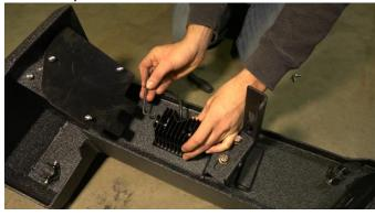
Loosely install the frame brackets onto the back of the bumper with a 15mm wrench, and 13mm socket using 4 of the included M10x35mm flange bolts. They will need adjusting later.
