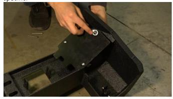
Install your backup sensors with a 3mm Hex Wrench. Again, these are location specific. Ensure they're installed into the same bracket location as the factory bumper.
