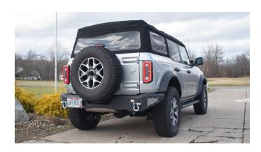
With the help of a friend, hold the bumper up to the frame rails and secure it by reusing your 4 factory bolts in the bottom of the rail, and the included M14 bolts into the side nutplates with an 18mm socket.
