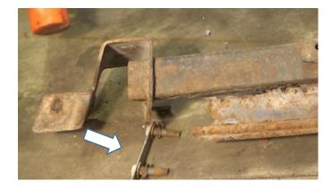
Set your new bumper on a flat surface facing away from you. Set the hitch onto the bumper's brackets and push the stud plates through both the bumper and hitch.
