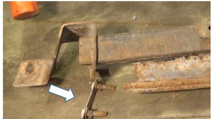
Set your new bumper on a flat surface facing away from you. Set the hitch onto the bumper's brackets and push the stud plates through both the bumper and hitch.
