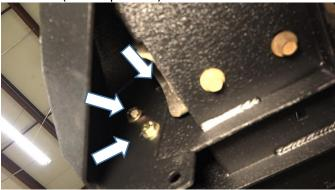
Shift the bumper around until it is centered and flush with the fenders.
