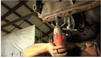
Loosely install the winch plate into those holes by reusing the factory bolts, and 4 bolts for the front of the brackets.
