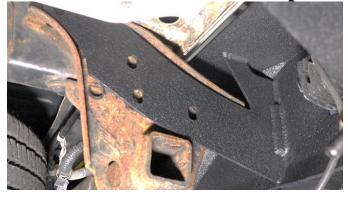
With the included 6 M12 Flange Hex bolts and a 19mm socket, install the bumper. If you have a hitch, 3 bolts will be used on each plate. If you do not have a hitch, only 2 will be used.
