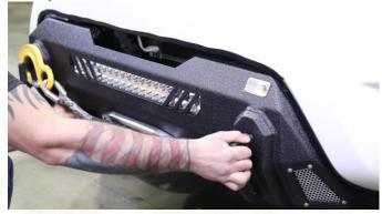
Shift the bumper left and right until it is centered. Once it is in place, tighten down the 6 nuts.
