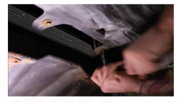
With a 10mm socket, remove the bolt below each headlight along the trim.
