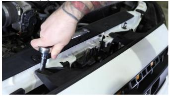
With a screw driver, remove the two top push clips just inside the grill. Gently and evenly tug at the grill and remove it from the vehicle.
