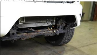
With a marker, draw a cut line around the corner of the valence so that it provides a flat surface for the rubber gasket to install on. Begin carefully removing the trim, and begin installing the Uchannel gasket along the cut line.
