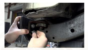
Insert a flat washer, lock washer, and 10mm bolt through the backing plate and into the rear bumper. **Do not fully tighten at this time.** You will need some room to move the bumper around as you install the other bolts. Repeat for all locations.
