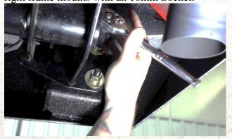
With the included tapered bolts, washers, lock washers, and nuts, secure the center of the bumper to the center frame mount.
