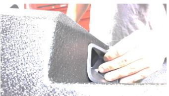
If your model has sensors, you will need to reinstall them into the Mako using the required Sensor brackets and bezels listed above, ensuring the each sensor returns to their 'one
