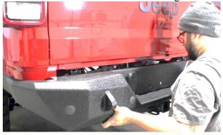
With the included flat washers, lock washers, and hex nuts, secure the bumper to the left and right frame mounts with an 18mm Socket.
