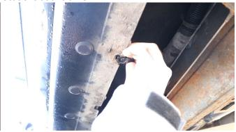
At the front of the vehicle on the passenger side, install the included upper bracket and bolt plate onto the vehicle, as shown, with a 13mm socket. Insert the stud through the clip.
