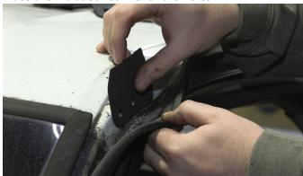
Install the side specific brackets with the included hardware. You can identify which side is which by the top flange pointing towards the front of the vehicle.
