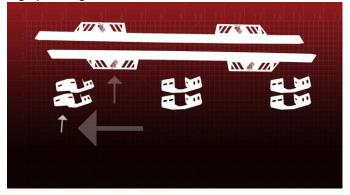
Secure each bracket with a 13mm socket.
