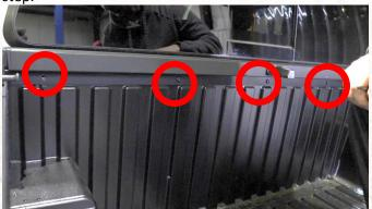
Next, with the remaining hardware, install the included stand-offs into the 5 upper holes of the panel so that the larger holes touch the plate, and the bracket pushes over the panel.
