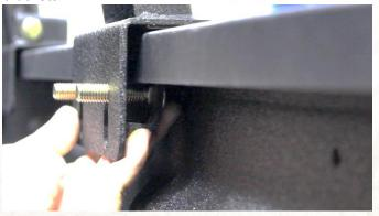
The 2 Arch brackets closest to the cab will require the included Spacers as the bed has a tapered shape and is wider at these points. Slide the spacer just behind the arch bracket, followed by the channel brackets.
