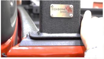
The arch with our signature plate in the center faces the rear. Spacing will be determined by the support braces.
