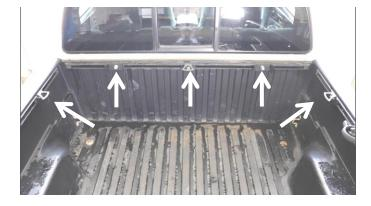
Determine the spacing needed for your gear and slide the T-Nuts as desired. Begin securing the brackets with the included hex bolts and washers with a 19mm socket.
