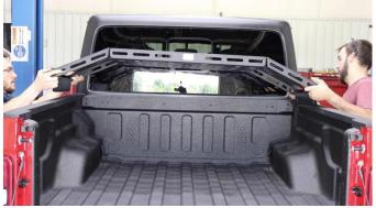
With a Steel Clamp, 2 carriage bolts, washers, lock washers, and hex nuts, insert the bolts into the Clamp as shown, and rotate it behind the Rack bracket and into place.
