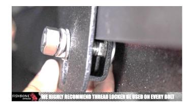
Push the Clamp high into the vehicle's rail, so that it grips the steel flange, and tighten down the bolts with a 19mm socket.
