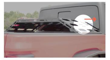
Using 6 of the included button head bolts, washers, lock washers, and hex nuts, loosely assemble the Side Plates to the Center Plate. They will be tightened in the last step.
