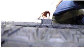
Completely tighten down the 3 hex bolts.
