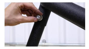
With the hub mount and frame, secure the two with 4 M12 bolts, 4 M12 washers, 4 oversized washers, 4 Nyloc nuts, and 2 19mm sockets.
