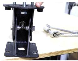
Hold the mount up to your tire and adjust its length so that the mounting plate is flush or near flush with the tire, ensuring that it will lie properly on the mount.
