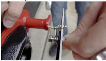
Secure each bolt with a 10mm socket and 4mm allen key.
