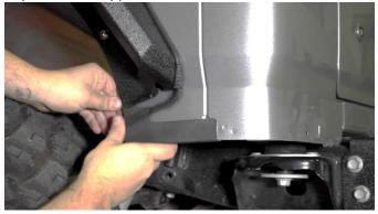
NOTE: If you would like to reinforce the guards positions onto the body, we've included 4 self-taping screws, two for each side, to be installed at the dimpled zones shown below.
