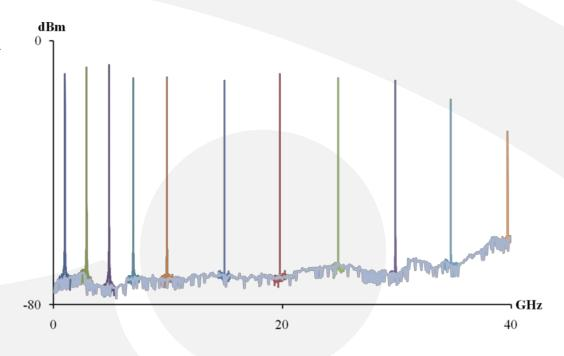
Sample heterodyne signals measured via photoreceiver and RF spectrum analyzer. High CNR observed. Characteristic shape demonstrated. Frequency response of Photoreceiver measured through compilation of heterodyne signals.
