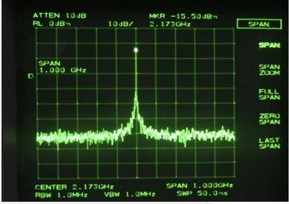
Sample Heterodyne signal measured via Photodiode and RF Spectrum Analyzer. High CNR observed. Characteristic Shape demonstrated.
