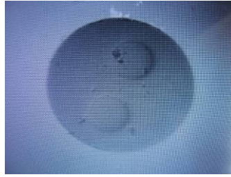
Dirty: Cleaning required
