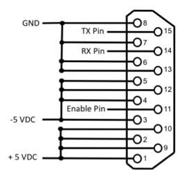
Pins 1, 2, 9, 10 - +5 VDC. It is important to have all pins connected for proper operation.
