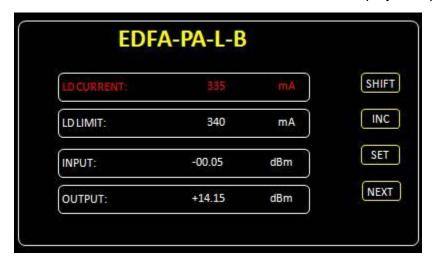
The Main Display allows the user to quickly view the various specifications of the EDFA-PA-L-B. By pressing the Next button, you can proceed to the next page. Follow the onscreen instructions to edit the various parameters.
