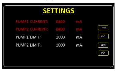
2. The SHIFT button on this page will move the cursor to next editable digit. The INC button will increase the selected digit by one for each press, after 9 the digit will cycle back to 0. Press the SAVE button to apply the new setting. Pressing the ESC button will return you to the main page.
