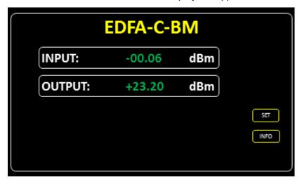
The Main Display allows the user to quickly view the input and output of the EDFA-C-B. Pressing the SET button will take you to the SETTINGS page and the INFO button will take you to the SYSTEM INFORMATION page (see next section).
