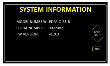
4. Pressing the UP or DOWN arrows will allow adjustment of the LCD backlight.
