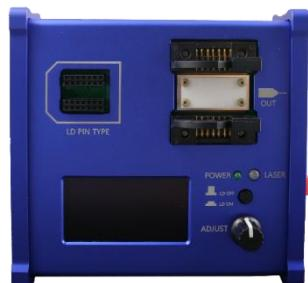
The Optilab Universal Laser Diode Controller (ULDC) is designed to drive DFB-1550A-PM and other 14 pin butterfly laser diodes. It provides a stable and precise current source up to 500 mA in ULDC-500-MC and 1000 mA in ULDC-1000-MC, along with temperature control and monitoring function to the laser.
