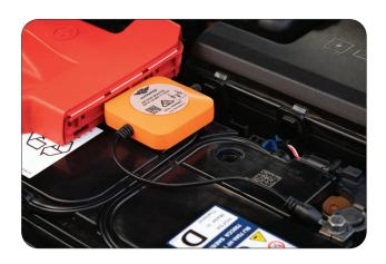
The Ultimate BM app is simple to use, and not only monitors battery voltage, but will run cranking and charge tests as well as including a trip function to monitor charging periods while you drive.
