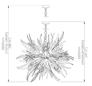
Due to its weight (51  $\!\!\!/\!\!\!/$  lb/23.2kg) this luminaire must be mounted or supported independantly of an outlet box
