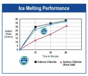
The tests were performed by the Swedish VTI by spreading 10 grams of each ice melter evenly over an icy surface at +21  $^{\circ}\text{F}.$
