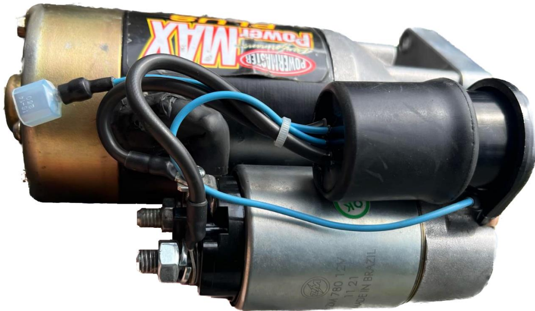
Powermaster starter motor with 12V Solenoid Control Relay attached
