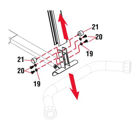
Take off the connecting sheet of rear stabilizer (4) and the U bracket will slide off (3).
