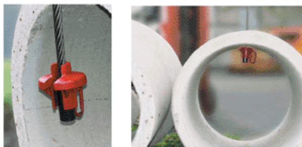
Once set, you are ready to lift the pipe.
