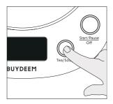
2.Press the "preset" button, the light will be on, the screen will display "preset", and the total standby time and cooking time will be displayed; Turn the "Time +/ --" knob to select the desired preset time.
