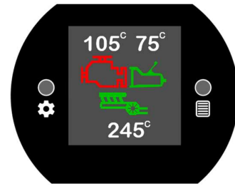
Alarm Flashing and Audible
