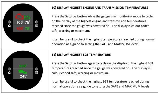
**To restore the gauge to factory default settings** - Press and hold the Settings button while the gauge is being powered on.
