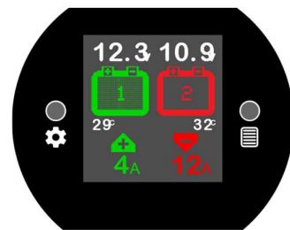
Battery 2 Low Voltage Alarm Flashing and Audible
