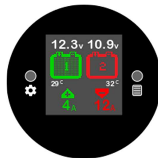
Battery 2 Low Voltage Alarm Flashing and Audible
