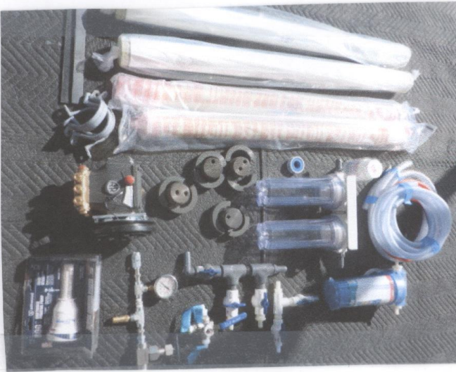
Typical Large Engine Driven 40GPH DualRO Watermaker
