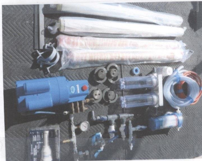
Typical 1½ HP dual RO membrane watermaker 40GPH Watermaker
