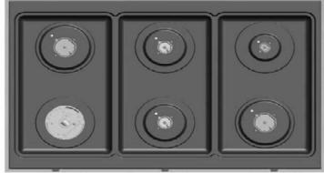
Dual Burner LPG: 1.27 - L20 NG: 2.38 - N21 Semi-Rapid Burner LPG: 0.95 - **L22** NG: 1.55 - **N22**  Rapid Burner LPG: 1.08 - L15 NG: 1.79 - N15
