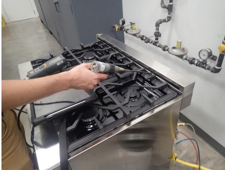
Figure A: This figure demonstrates a proper sampling location. The gas range oven cavity vents itself out through flue vents located behind the left or right side of the top burners of the stove top.
