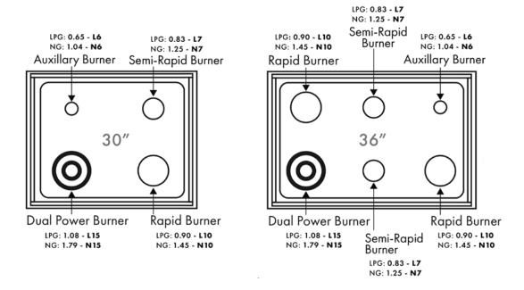
Reference the diagrams below if your drop-in cooktop was manufactured after June 2021. To check, reference the rating label on the underside of the product.
