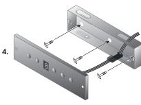
4. Mount the control panel by securing it with three screws through the back of the panel into a nearby wall or cabinetry. Depending on your preferred placement, you may secure the panel with screws into the top and/or bottom perforated holes. NOTE: Every installation will be unique depending on the house and mounting preference.
