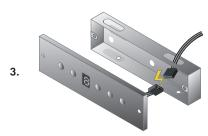
3. From the inside of the range hood, disconnect the 9-pin connection cord from the existing button panel, filter the cord through the perforated hole, and then connect to the cord on the control panel.
