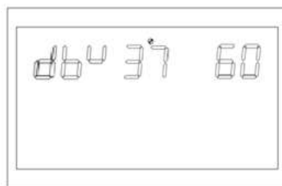
Figure 1-45 Battery dual-way output low-voltage shutdown point page
