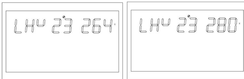
Figure 1-33 Setting high voltage point of grid
