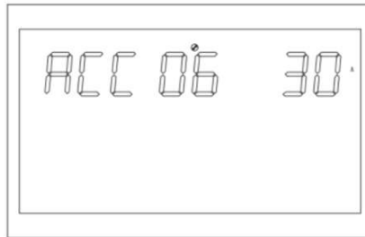
Figure 1-17 Setting the grid maximum charging current
