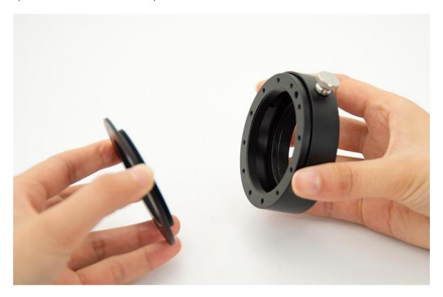
3) Mount the M54 filter drawer on the camera via threads.
