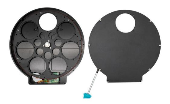
3) Disassemble the filter wheel carousel (Note: Please do not disassemble or move the central screw of this carousel, otherwise the EFW will be damaged)
