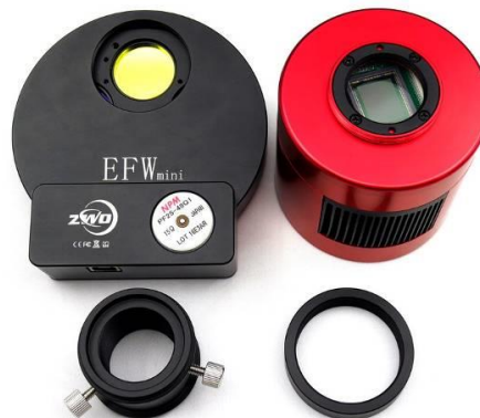
Screw off the T2-1.25" holder on the EFW, screw off the T2 ring on the 1600 camera.
