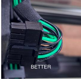
A Note About **Strain Relief**: The best we can do is ensure that each wire has neutral forces on it to the best of our ability. Molex recommends strain relief be approximately 2cm from the end of the 14-pin Microfit 3.0 connector. The toolhead and pcb designs do not accommodate appropriate strain relief, so we do the best we can
